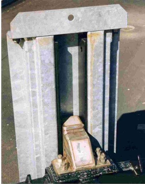
**Figure 9. Slide Guide Current Design Detail (Note hole at top of wear strip to aid removal)**
