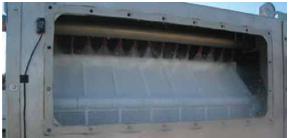
Low pressure water jets for effective cleaning
