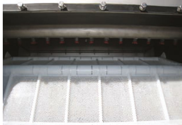
Patented mesh panels eliminate the problem of hairpinning and blinding found with other band screens
